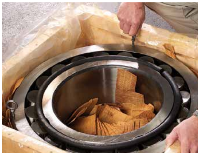
Fig. 2. Eyebolts can be inserted into lifting holes.
