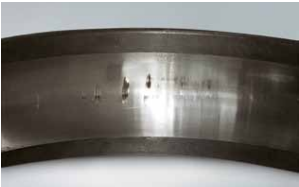
Photo 12.2 Part: Outer ring of Photo 7-12-1 Symptom: False brinelling occurs on the raceway Cause: Vibration from an external source while stationary
