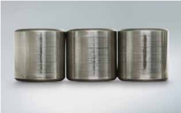
Photo 12.4 Part: Rollers of a cylindrical roller bearing Symptom: False brinelling occurs on rolling surface Cause: Vibration from an external source while stationary
