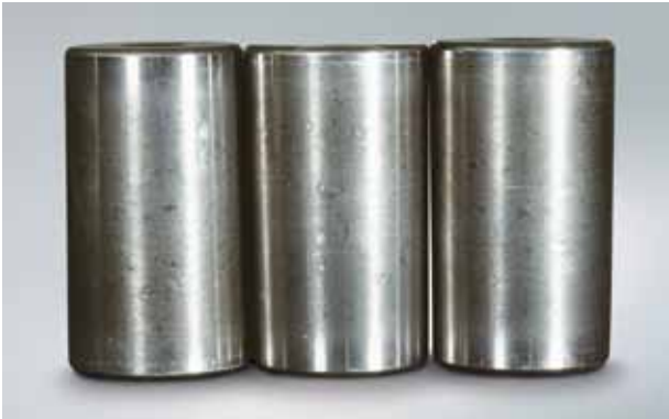
Photo 8.4 Part: Tapered rollers of Photo 7-8-3 Symptom: Small and large indentations occur over the rolling surface Cause: Debris caught in the surface
