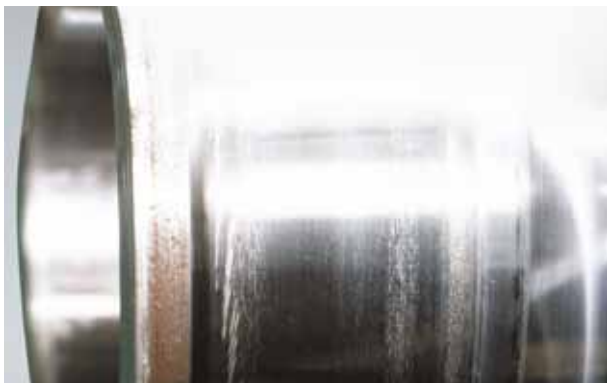
Photo 4.5 Part: Inner ring of a spherical roller bearing Symptom: Partial smearing occurs circumferentially on raceway surface Cause: Poor lubrication
