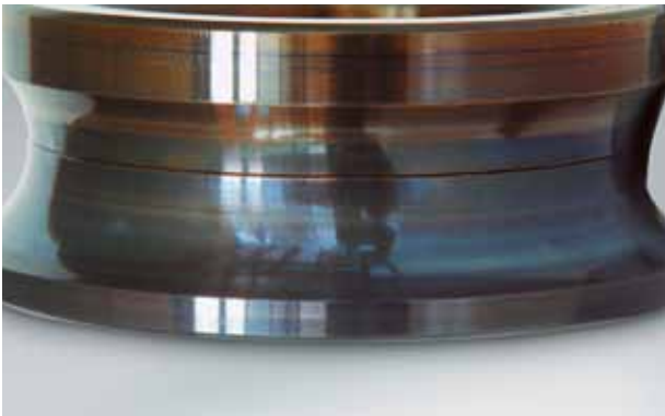
Photo 18.2 Part: Inner ring of a 4-point contact ball bearing Symptom: Bluish or purplish discoloration on raceway surface Cause: Heat generation due to poor lubrication
