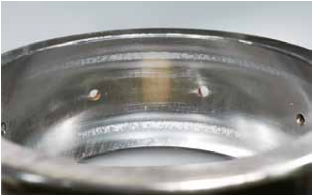
Photo 2.4 Part: Outer ring of a spherical roller bearing Symptom: Peeling occurs near the shoulder of the raceway over the entire circumference Cause: Poor lubrication
